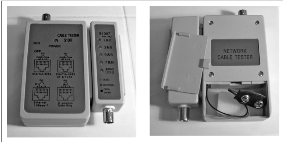
Figure 5-9 Cat5 cable testers.
